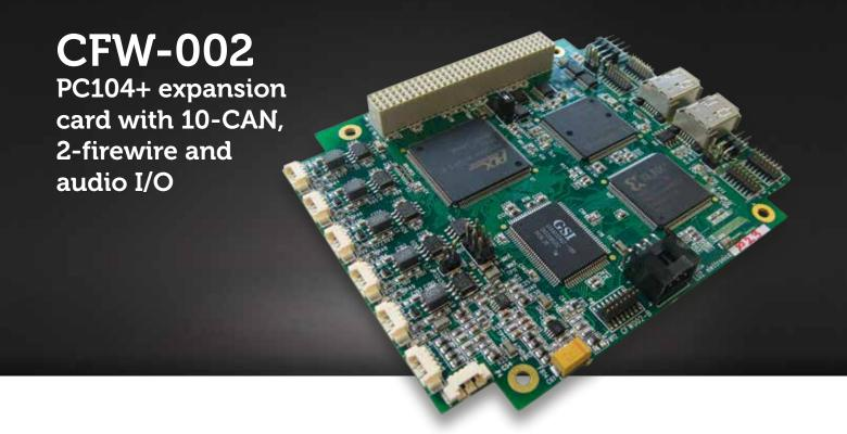
The CFW-002 board is PC104+ standard expansion card directly connected to the PC104+ bus. The board has 10 CAN Bus 2.0B links, 2 IEEE 1394 (Firewire) high speed ports, one stereo microphone preamplifier and a single D-Class speaker output.
